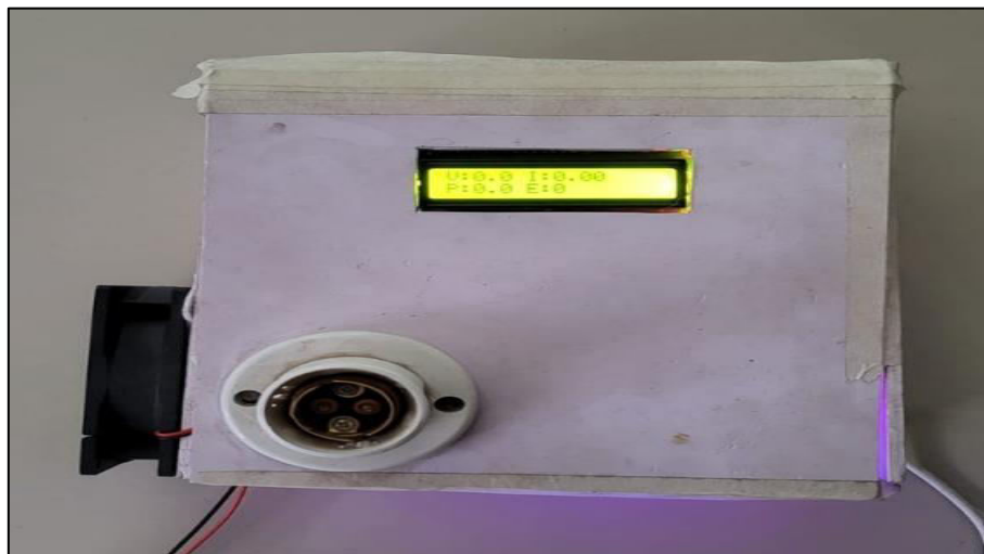
FIGURE.3. FABRICATED PROTOTYPE OF THE PROPOSED SMART ENERGY METER
